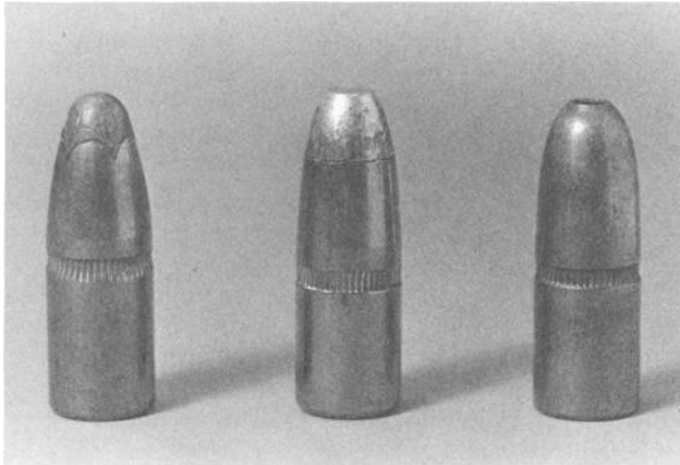
FIG. 1—(Left to right) Soft-point, Silver-tip, and hollow point .30 caliber hunting bullets.
